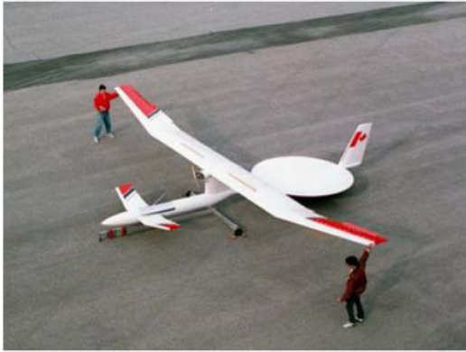
Fig. 8. Stationary High Altitude Relay Platform (SHARP) airplane, having a large rectenna behind the wings, allowing for power to be transmitted to it from the earth, and thus is able to stay in the air for long periods of time, potentially months
