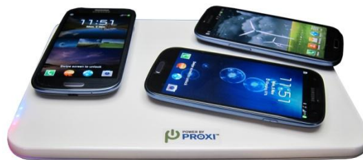
Fig. 4. A device by Powerbyproxi, charging multiple mobiles wirelessly simultaneously
