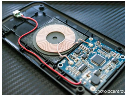
Fig. 13. Inside look of a phone enabled for wireless charging
